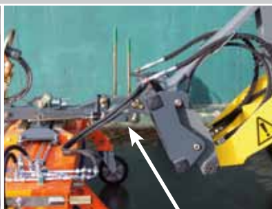
Yard loader / Front loader attachment with parallelogram and pendulum compensation incl. height indicator
