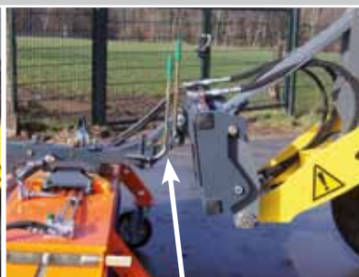
Yard loader / Front loader attachment with parallelogram and pendulum compensation incl. height indicator
